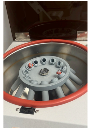
Figure 2: Loaded swivel head centrifuge with SST tubes.
