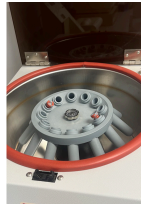
Figure 2: Loaded swivel head centrifuge with SST tubes.
